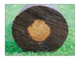
The main objective of pole treatment at the OTDS plants is full penetration of the sapwood, no matter how thick it is.
